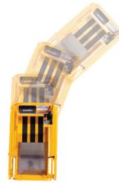
Spin – Machine rotation **without** forward or reverse movement, moving directly left or right.
