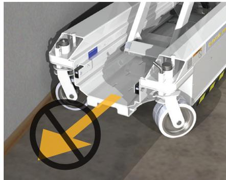
In this situation do not use forward motion, as this will cause the machine to make a sharp turn toward the wall.
