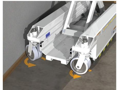
Instead, use spin to rotate the casters away from the wall before traveling
