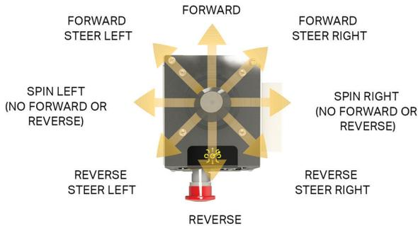
Understanding the difference between Spin and Turn on the Hy-Brid HB-830/HB-1230 is essential for proper machine control and avoiding unwanted caster movement.
