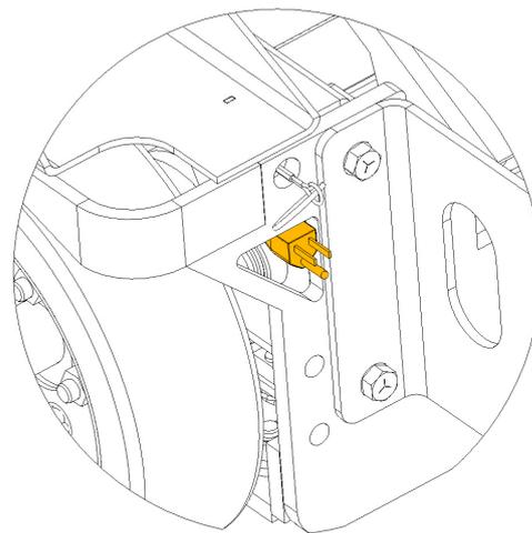
FIGURE 24: Power to platform plug
