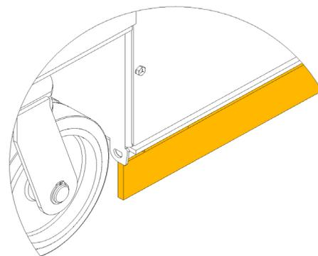
FIGURE 3: Pothole Guard
