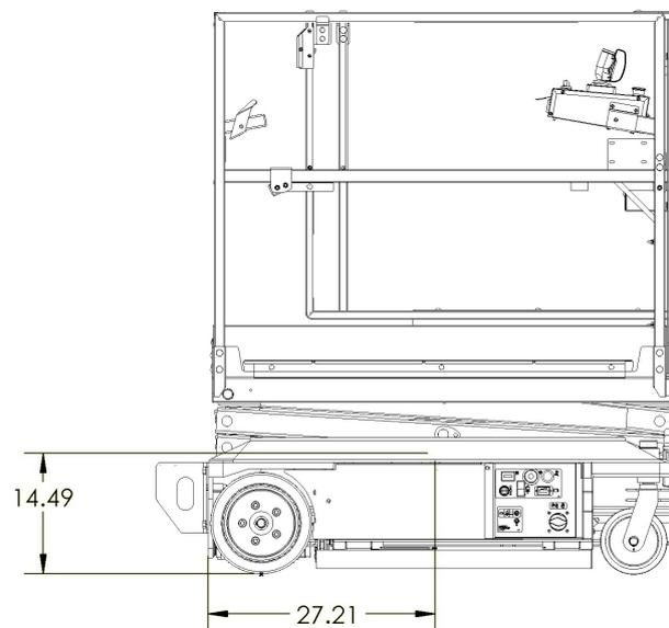
FIGURE 15: Center of Gravity
