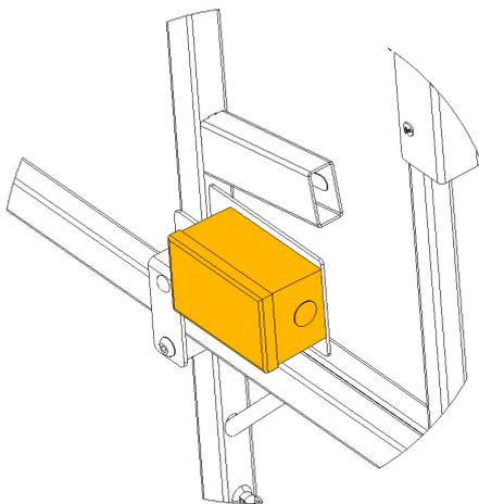
FIGURE 23: Power to platform outlet
