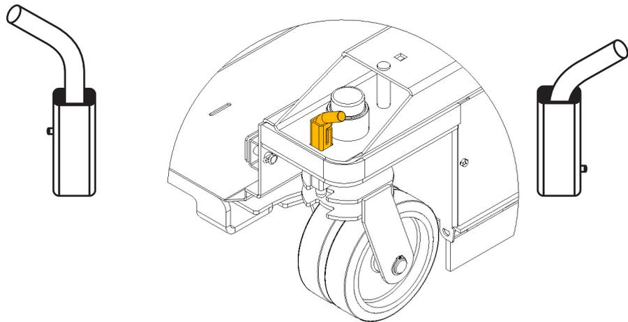
FIGURE 11: Caster Lock engaged
