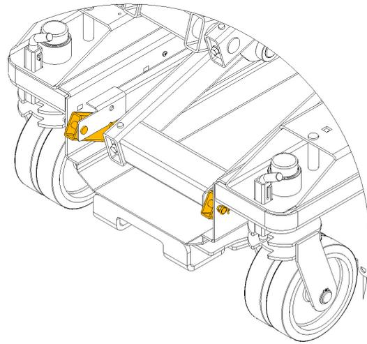
FIGURE 7: Maintenance Lock In Use
