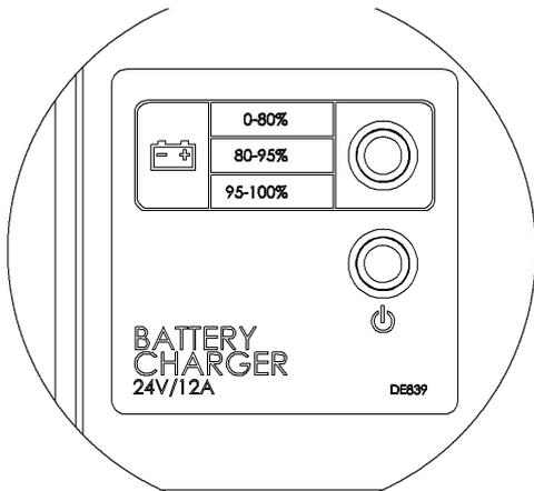
FIGURE 26: Battery Charger LED Display
