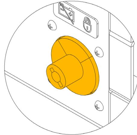
FIGURE 20: Master Power Switch Knob Removed
