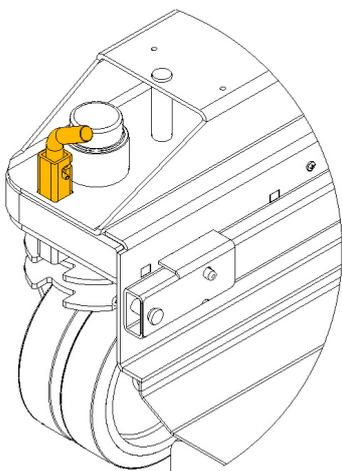
FIGURE 10: Caster Lock Disengaged
