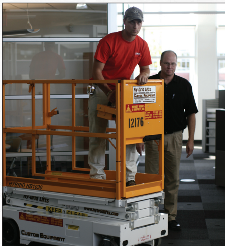
The Custom Equipment Hy-Brid HB1030 scissor lift is light enough to ride over access floor panels at Bick Group's headquarters.
