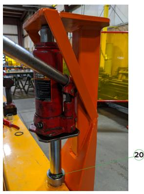
21. Using steady pressure, pump the bottle jack and push the DU bearing in until it is seated flush.
