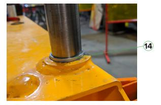
15. Remove the bottle jack, allow the DU mandrel to rest on the lower DU bearings in the steering bushing, and remove and replace the jack frame in the up position.
