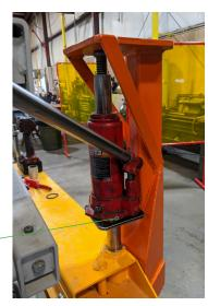
17. Using steady pressure, pump the bottle jack and push the DU bearings out of the bottom of the steering bushing. There will be a total of (2) bearings.\*
