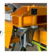
Inspect the caster shaft and DU bearings inside the steering bushing for abnormal wear. If the DU material is depositing onto the caster shaft, this is an indication that the DU bearings have been compromised and should be replaced.
