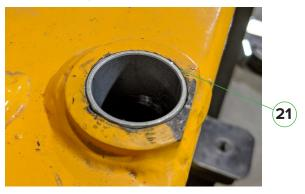
22. Place the jack frame in the down position. Set the fresh DU bearing (HARD-001) straight into the bore of the steering bushing. Place the DU Install Long into the DU. Place the bottle jack on the jack frame and under the DU Install Long.
