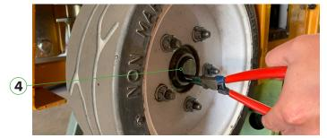
Remove locking cotter pin from steering clevis using needle nose pliers.
