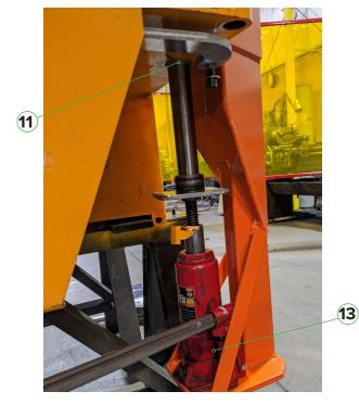
14. Using steady pressure, pump the bottle jack and push the DU bearing out of the top of the steering bushing. There will be a single bearing.
