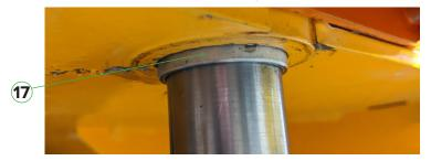
\*With the top DU out, in rare cases the bottom DU's may not extract using the mandrel and hydraulic pressure. If this is the case, the DU punch may be inserted from the top and a heavy steel hammer used to drive out the 2 lower DU bearings.
