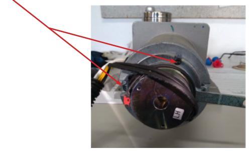
2. Remove 2 nuts holding brush end housing
