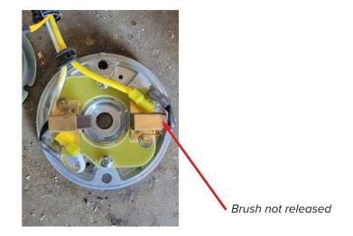
4. Release the brush by relieving the coil spring tension.
